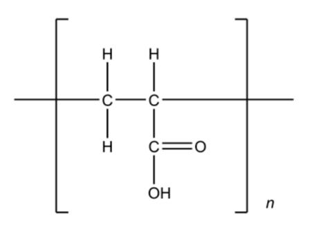
Acrylic acid monomer unit in carbomer polymers.
